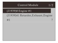
4. After enter the system, users can read ECU information, read fault code, erase fault code and live data. If it indicates "communication failure" during the diagnosis, please check whether the key switch is turned on, selected diagnostic protocol is right and vehicle diagnostic socket has signal voltage, etc.
