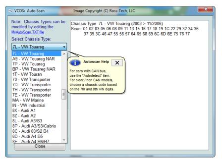
Important! AutoScan is probably the single most important function in VCDS. We recommend that you run and SAVE a complete AutoScan on every single vehicle that you work on. This will give you a history of the vehicle that can be invaluable in the future, for example if an ABS module fails and needs to be replaced. Referring back to earlier Coding is often MUCH simpler than trying to figure out such values from scratch.
