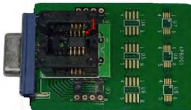
Picture 4: Pin 1 position on the clamp
