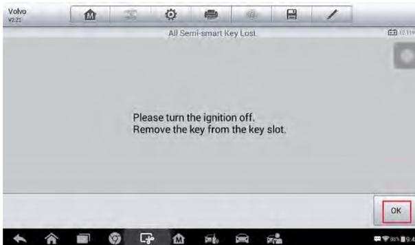
**Figure 21 Sample All Semi-smart Keys Lost Screen 13**
