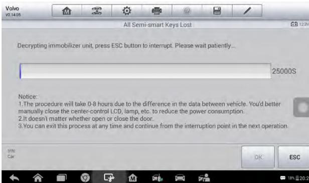
**Figure 14 Sample All Semi-smart Keys Lost Screen 6**
