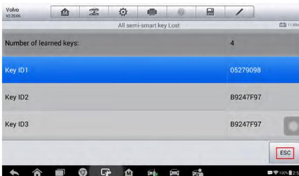
**Figure 22 Sample All Semi-smart Keys Lost Screen 14**
