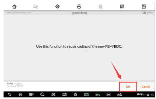
Figure 34 Sample Repair Coding Screen 2
