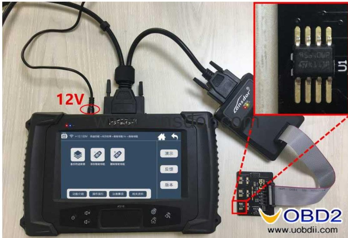
**Note:** If you can not read data with the KPROG adapter, you can use a programmer to read and copy the data into the K518ISE specified folder, the path: K518 -> file -> feature\_553
