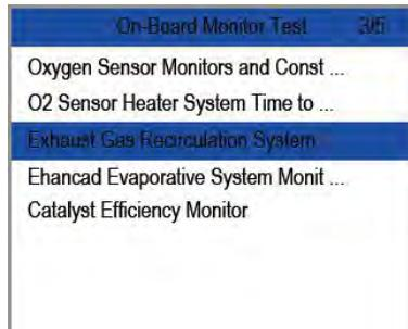
3. Use the **UP/DOWN** key to highlight a test group and press the **OK** key to confirm. A screen with details of the selected sensor displays. Use the up and down arrow keys to scroll through data to select lines, and left and right arrow keys to scroll back and forth through different screens of data.
